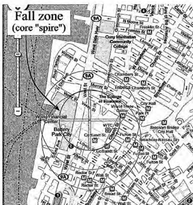
Figure 125. The minimum estimated distance remaining core columns would have reached had they fallen over. 6
