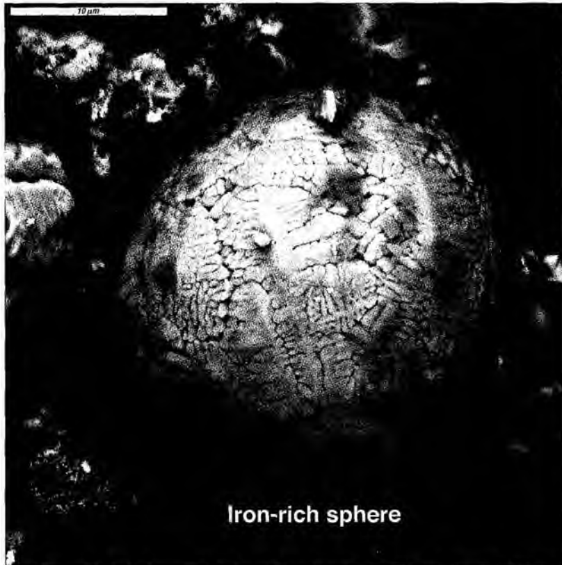
Figure 347. (10 \mu m - scale) Iron-rich sphere found in dust from the WTC. Using the scale on the image, the diameter of the iron-rich sphere is about 25 \mu m. http://pubs.usgs.gov/of/2005/1165/graphics/IRON-04-IMAGE.jpg 27
